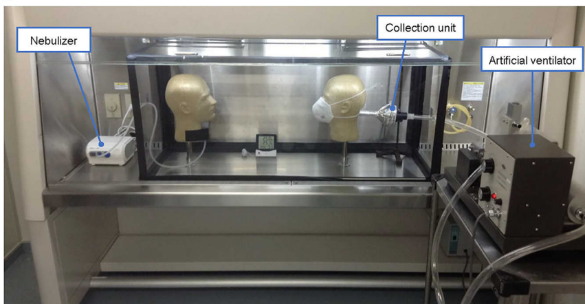
FIG 1 Simulation system for airborne transmission of virus droplets/aerosols. Schematic image (A) and a photograph (B) of the system. A test chamber for airborne transmission experiments was constructed in a BSL3 facility, and two mannequin heads were placed facing each other. One mannequin head was connected to a customized compressor nebulizer and exhaled a mist of virus suspension through its mouth to mimic a viral spreader. The other mannequin head was connected to an artificial ventilator through a virus particle collection unit. Tidal breathing, conducted by the artificial ventilator, was set to a lung ventilation rate representative of a steady state in adults (i.e., 0.5 liter of tidal volume, a respiratory rate of 18 breaths/min, and a 50% gas exchange rate). Face masks were attached to the mannequin heads according to each manufacturer's instructions.
